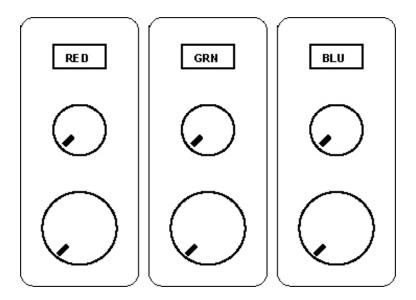
Each of the three colors can be controlled independently, using a control cluster that is comprised of a button and two knobs.
